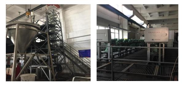
Figure 13: Hunan Research Facility spiral and flotation circuits
