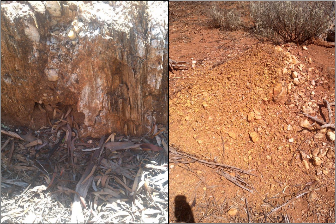
Figure 12: Left-hand side view north of costean wall cutting sub-vertical mylonitic contact between Amphibolite and Granodiorite with boudinaged quartz veins. Right-hand side spoil from a trench with altered granitoid and quartz vein.
